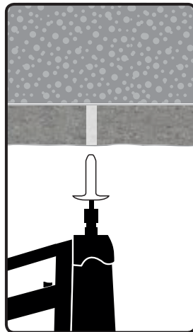
Locate the pre-positioned hole in the insulation sheet Insert fixing into position.
